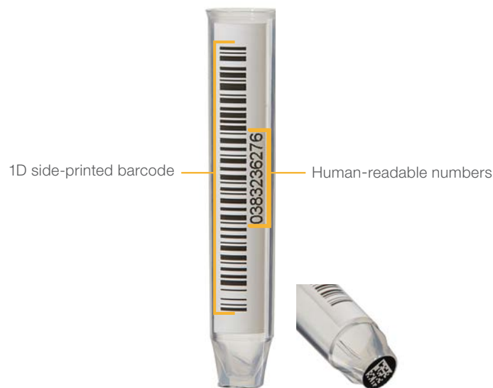
Figure 1. Image of a 1D side-printed barcode that matches the 2D barcode on the bottom of the tube.
